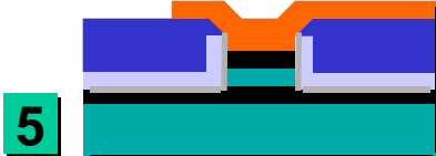
5 Planarization with Polyimide, Deposition of Contact Pads
