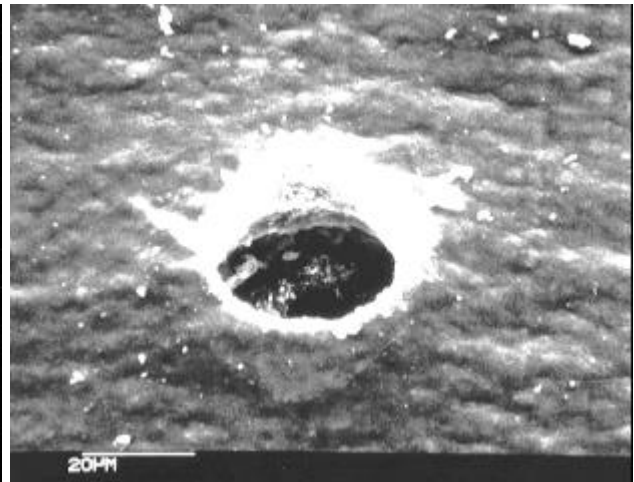
Fig. 13 Exit side of an EV strike on silicon carbide grain coated on a 0.001" thick aluminum foil.
