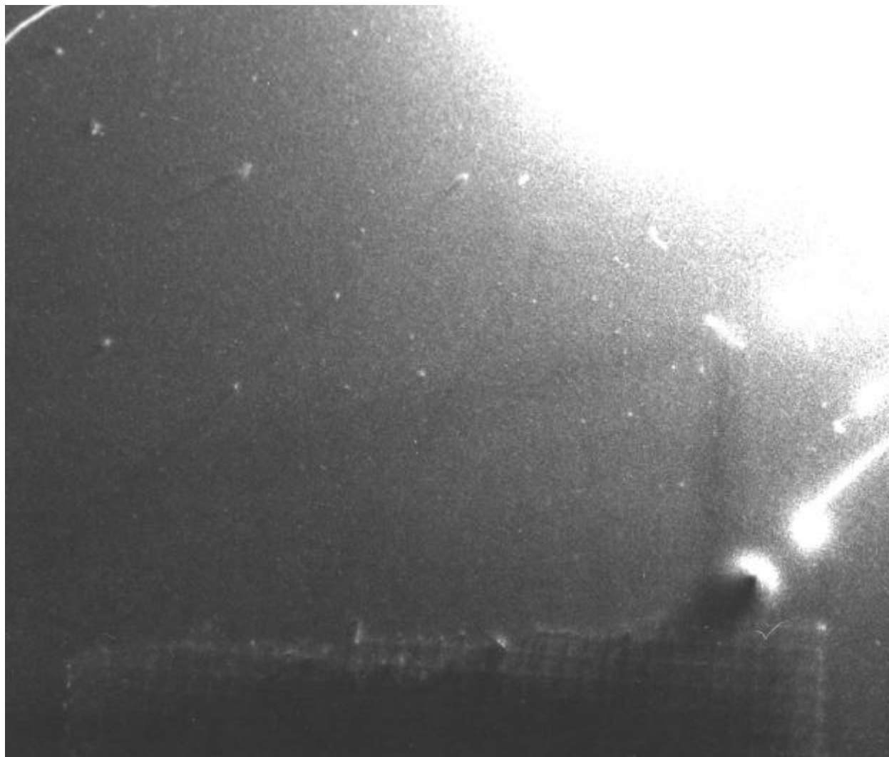
Fig. 18 Magnified view of region #2 in Fig. 15. The lower portion shows an image of the 200 mesh screen used. Many dust specks cast a sharp shadow from the point light generated by EV acceleration.
